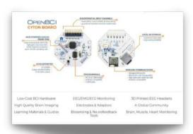
There are 8-channels in the Cyton Biosensing Board in which individual sensors are connected to these channels. These signals are displayed on the monitor. Further, we can apply Machine learning Algorithms to these signals, and hence this process makes the brain signal perform some specific tasks or control some equipment.
